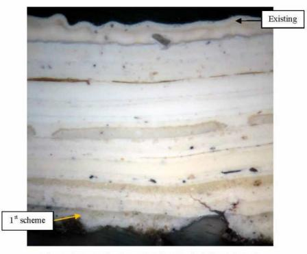
Photomicrograph of BIC/13 (x 200 digitally reduced) Building 89: South front. R/H lower window cill
